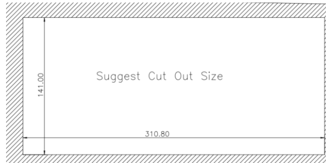
Figure 3-7: DM2-UW123J(L) Cutout Dimensions (Unit: mm)
