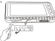
Note: For the very first time using, we recommend you charge with the AC adapter. Charging from PC's USB port will take 6 hours or longer.
