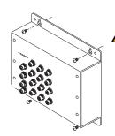
Instead of screwing the screws in all the way, it is advised to leave a space of about 2mm to allow room for sliding the switch between the wall and the screws.
