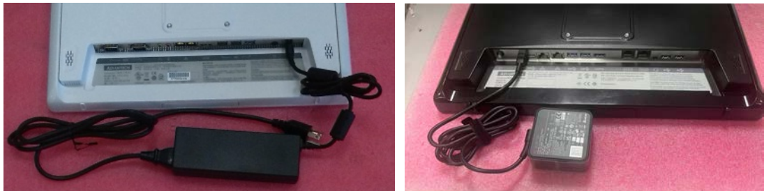
Figure 2.3 Power Cord to DC Input (Left Picture: UTC-320D/F/G/H/I, Right Picture: UTC-320K)
