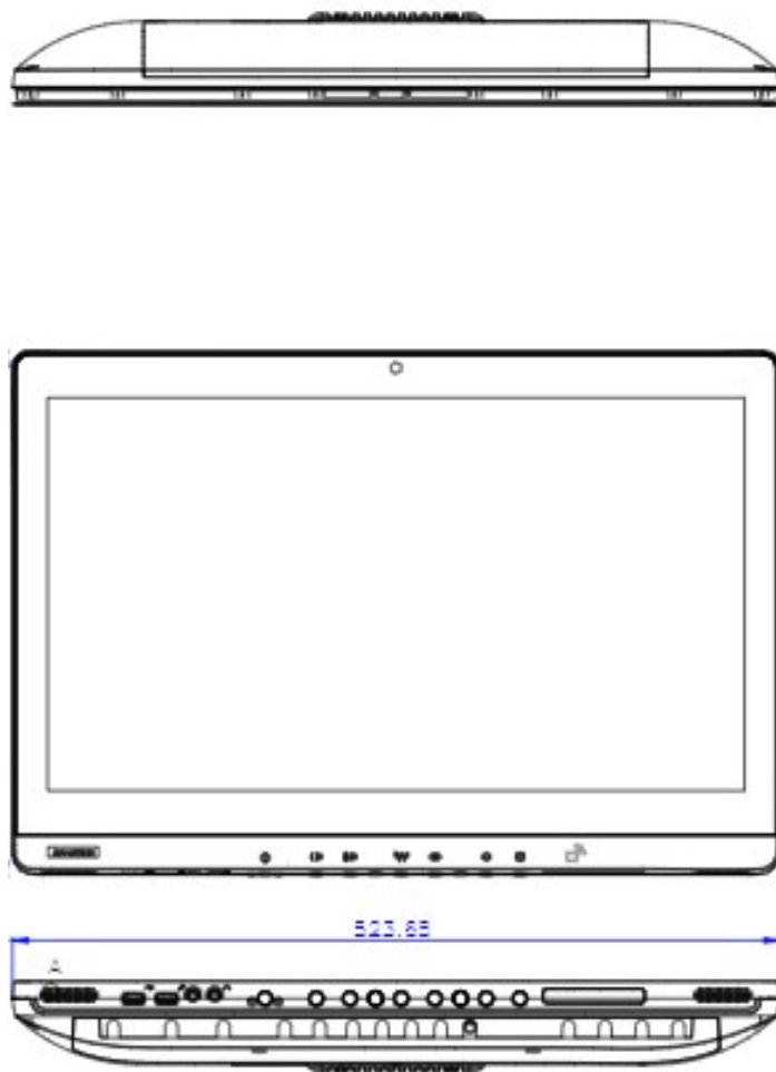
Figure 1.2 Dimensions of the POC-624-02 Series Device with Smart Card Reader
