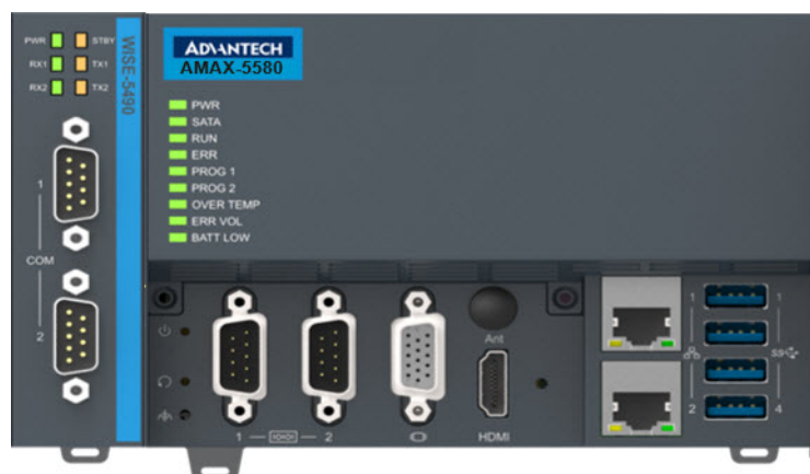
Figure 3.3 AMAX-5490 Serial Expansion module installation example
