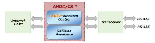
Auto Hardware Direction Control (AHDC™) technology makes it easier to manage 2-wire RS-485 half-duplex communications, eliminating the need for software interference. User does not necessary to write extra code for Windows applications to control the half-duplex protocol. Auto Hardware Direction Control (AHDC™) technology is the key feature of SUNIX UART, and this function is default enabling.
