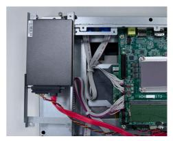
Screw in the four screws provided in the package to secure the SSD tray in place.Connect the SATA cable and the SATA power cable to SSD and the board connectors.
