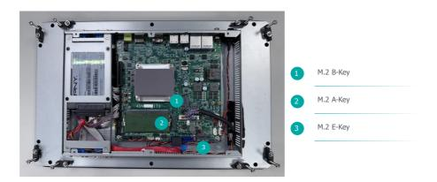
Before installing the M.2 module into the M.2 socket, please make sure that the following safety cautions are well-attended.
