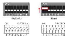
Manufacturer default jumper setting is OPEN (disable 120ohms termination resistors across the two wires)
