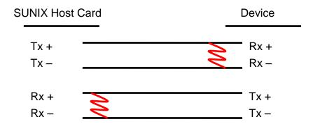
2-Wire RS-485 working model with termination resistor:
