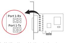
RS-422 or 4-Wire RS-485 working model with termination resistor:
