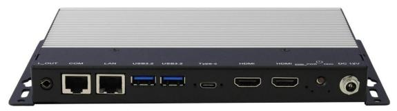
The image shows the function of the connectors and buttons as indicated by the text on top of the connectors, (starting from the left) including L\_OUT, COM, LAN, USB 3.2, USB 3.2, Type-C, HDMI, HDMI, EDID, PWR, HDD, and DC 12V.
