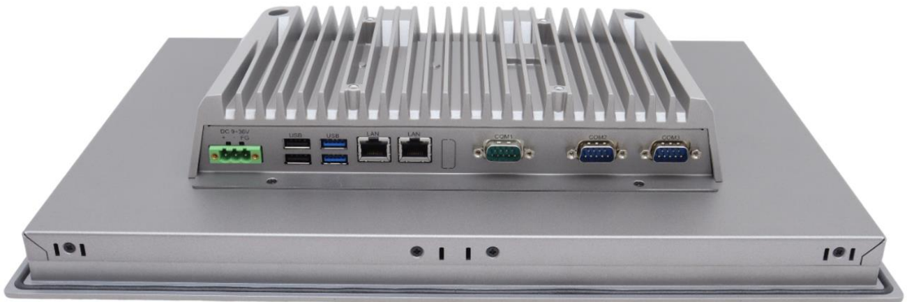
Figure 12 Rear View of ARCMHI-S-916D
