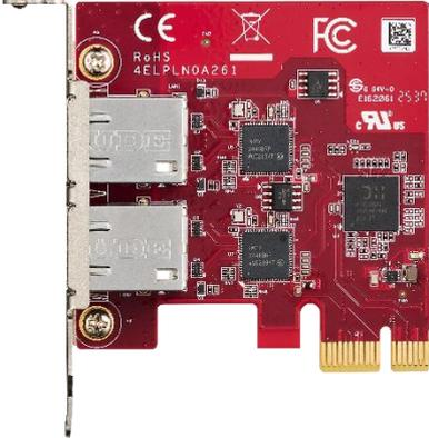
Figure 2: Low-Profile Bracket PCIe Board Picture
