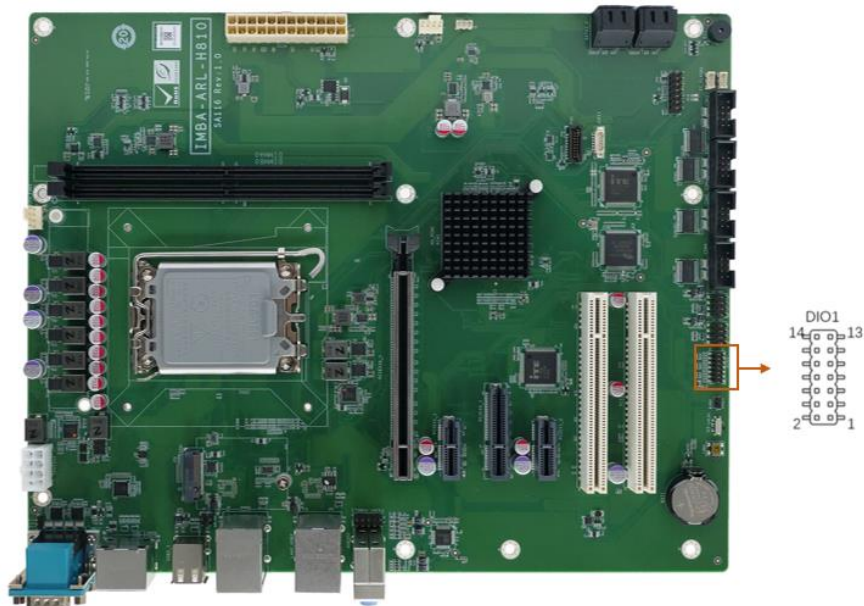
Figure 3-11: Digital I/O Connector Location
