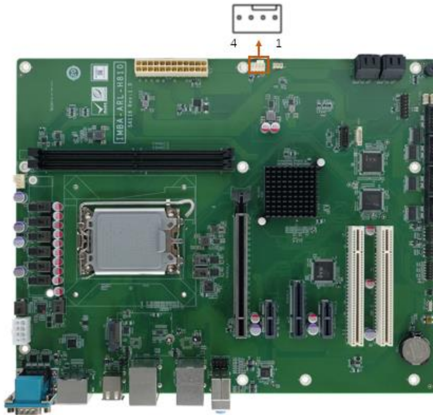
Figure 3-13: System FAN1 Locations
