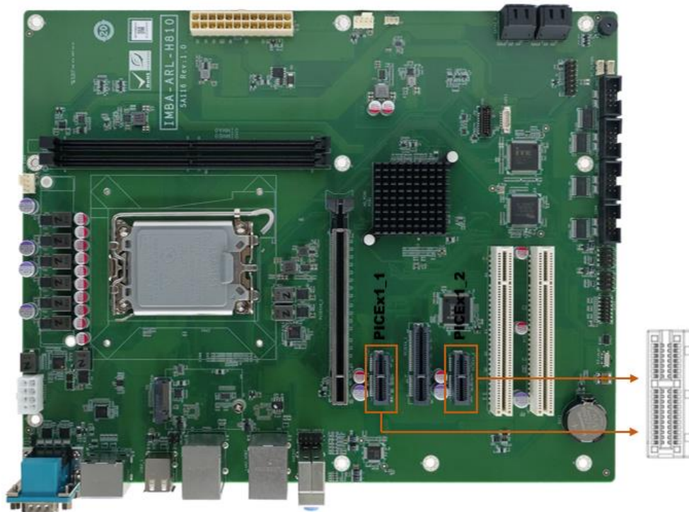
Figure 3-24: PCIe x1 Slot Locations
