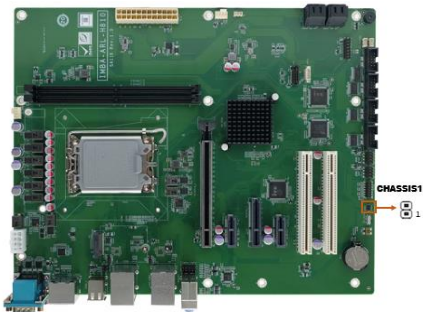
Figure 3-9: Chassis Intrusion Connector Location
