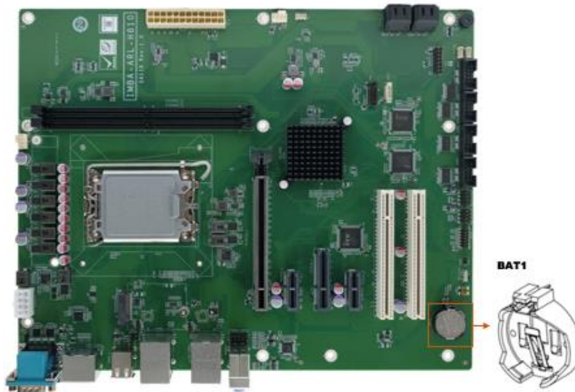
Figure 3-8: RTC Battery Connector Location
