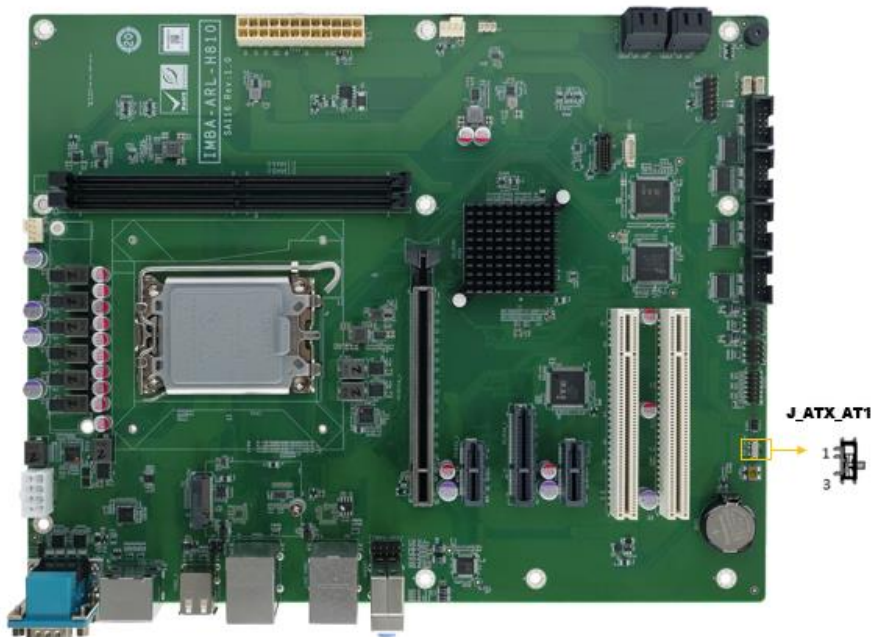
Figure 3-3: AT/ATX Power Mode Switch Locations
