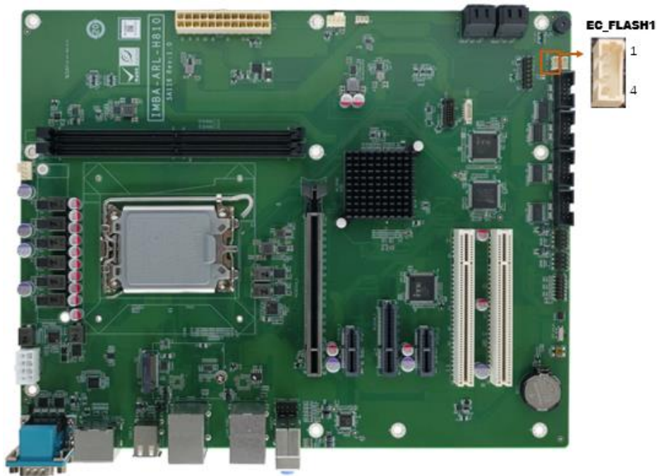
Figure 3-5: Flash Description Security Override Connector Location
