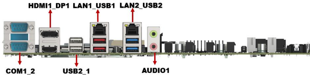
Figure 3-27: External Peripheral Interface Connector
