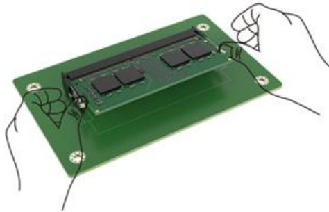
Figure 3-2: Open the handles of the Memory Slot
