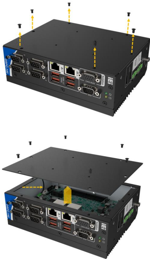
Figure 3-1: Remove the Cover
