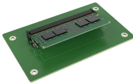
Figure 3-3: Insert the Memory Module
