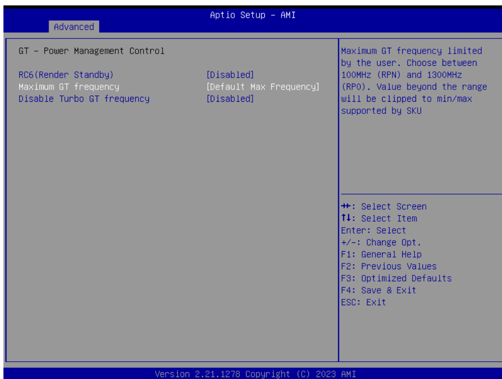
Figure 4.12 GT – Power Management Control
