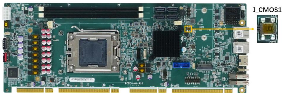
Figure 4-2: Clear CMOS Jumper Location
