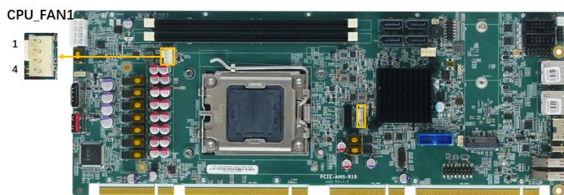
Figure 4-7: CPU Fan Connector Location
