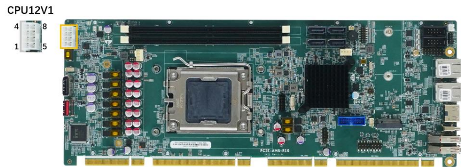
Figure 4-10: CPU 12V Power Connector Location
