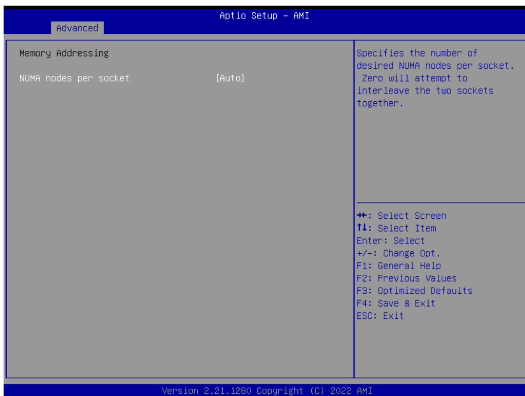
Figure 3.10 DF Common Options - Memory Addressing Screen
