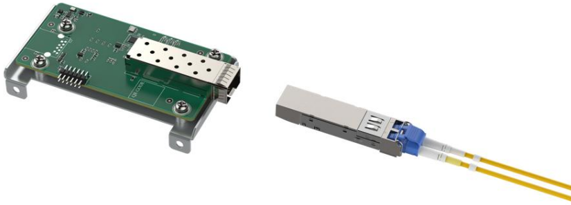
Figure 3-13: Connect the small card
