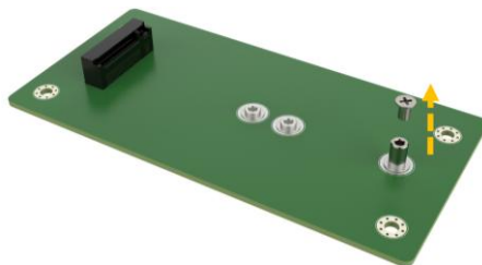
Figure 3-5: Remove the Retention Screw
