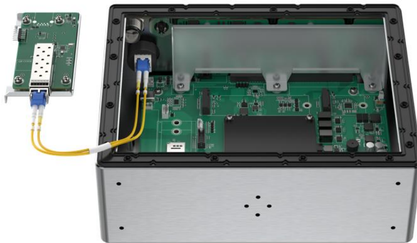
Figure 3-14: Connect the IO optical fiber port
