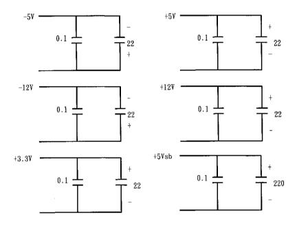
0.1 uf is ceramic, the other is tantalum. Noise bandwidth is from DC to 20Mhz
