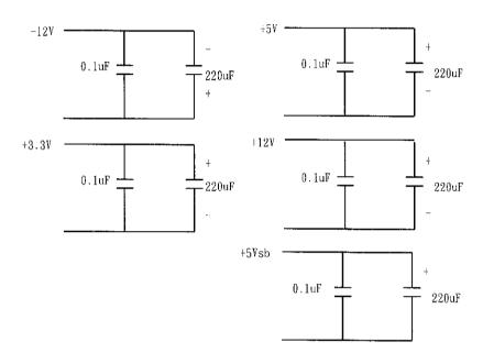
0.1uf is ceramic, the other is electrolytic capacitor. Noise bandwidth is from DC to 20Mhz
