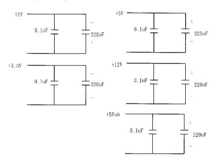
0.1 uf is ceramic, the other is electrolytic capacitor. Noise bandwidth is from DC to 20Mhz
